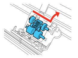
7. To install the new lower pickup roller, align the notches on the roller and slide it to the left.
